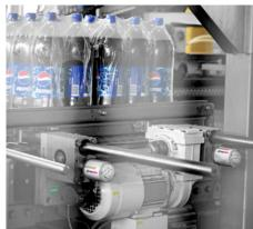
The bearing on the gear box is lubricated with two  $60\,\mathrm{ml}$  simalube lubricators.
