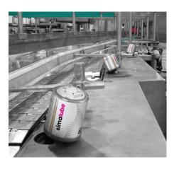
A filling line is equipped with several simulube lubricators.
