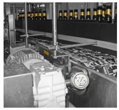
Lubrication of a transport belt with a simalube lubricator.
