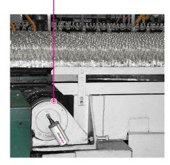
Lubrication of a conveyor belt drive.
